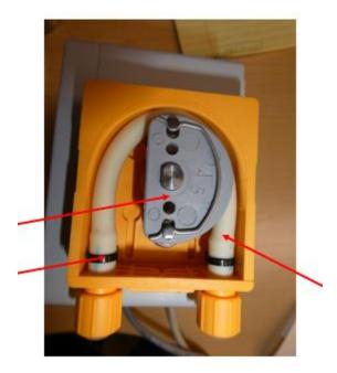
3) Once hose is removed wash and rinse out with white vinegar and massage kink out of affected area, reassemble and return to service.
